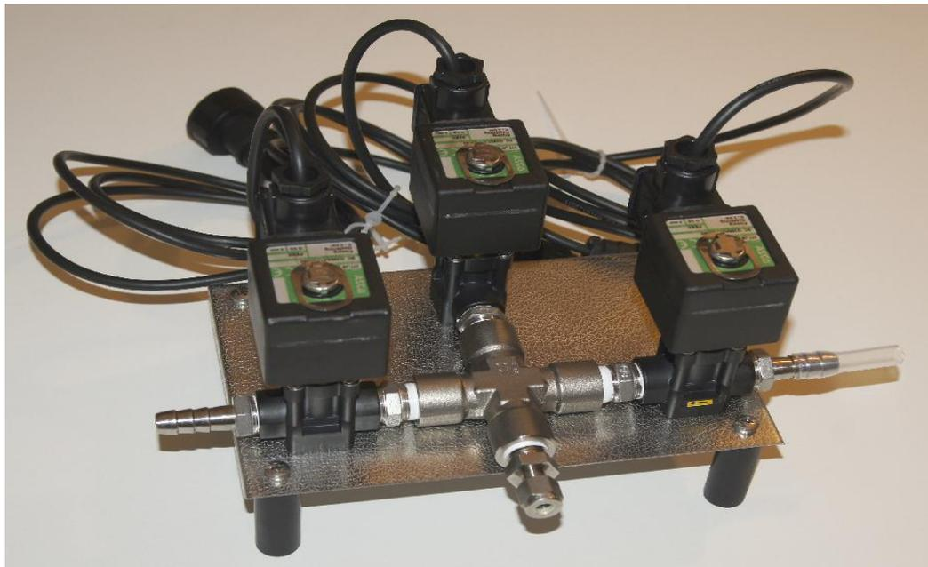
Fig. 11: Gradient valves
