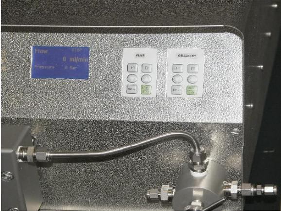
Fig. 10: Pump and gradient keyboards
