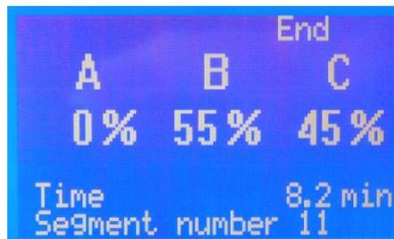
Another possibility how to stop gradient is to press the START / STOP button anytime during the run. Pump is running, delivering composition which was on the screen at the moment of STOP action. Next (third) pressing the START / STOP returns composition to the default gradient composition (gradient segment 0).
