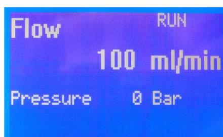
Then is possible pressing the START / STOP again to stop the pump. The pump motor starts stops rotation stepwise during approx. 4 s.
