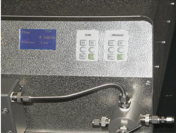
Fig. 10: Pump and gradient keyboards
