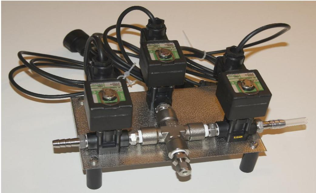
Fig. 11: Gradient valves
