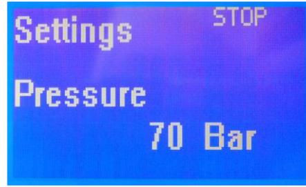
After switching on the pump is set to display the first item. In the upper right corner shows the status of the pump (at this moment, STOP). The display shows the current flow and the current pressure. After pressing the F1 key to get to the second operating item display, where it is displayed as the current primary pressure and secondary current flow.
