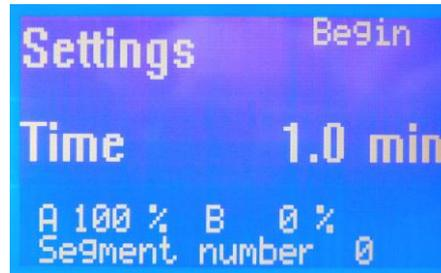
the value of B and C so that anytime is true  $A + B + C = 100$ . Taking the first gradient step, C is assumed to be  $C = 0$ , thus regulating the gradient of B. After pressing ENTER the instrument shall be recorded in all three gradient values A, B and C.
