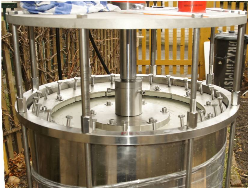
Fig. 14:: Upper piston ring installing
