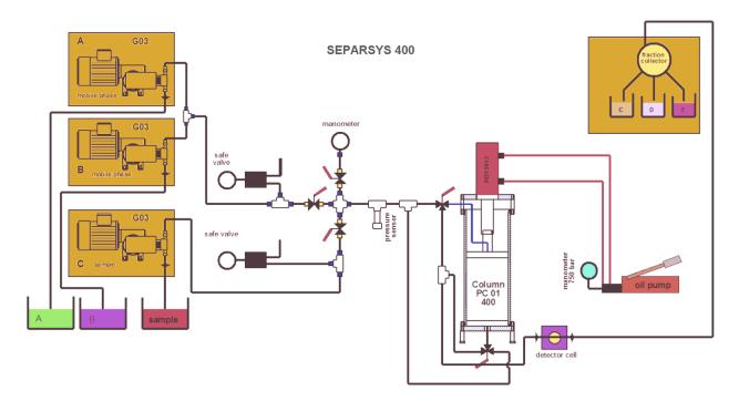
**Separsys 800 FP** is an industrial unit for liquid high efficiency, high pressure preparative chromatography. It can be used for isocratic, high pressure, high performance chromatography. It is completely controlled by modified **ECOMAC** software only. The unit consists of (see schematic drawing):
