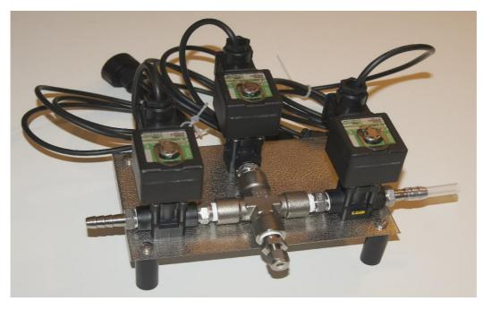
Fig. 11: Gradient valves
