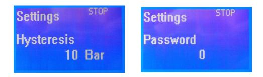
After checking the set of valuesis possible by pressing F2 to return to the default item and we can start the pump by pressing the START / STOP. After pressing the change in the upper right corner is visible (to RUN) and the pump starts to pump. If not, it is possible that the pump is blocked by one of the following reasons.
