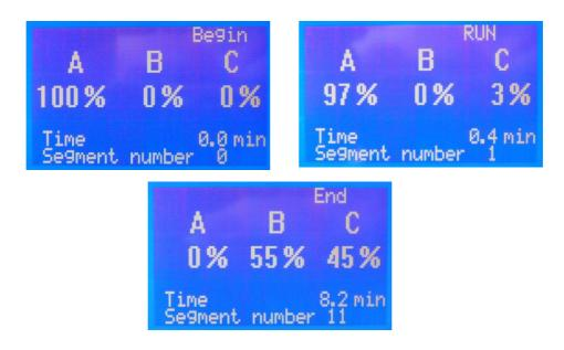
Another possibility how to stop gradient is to press the START / STOP button anytime during the run. Pump is running, delivering compostion which was on the screen at the moment of STOP action. Next (third) pressing the START / STOP returns composition to the default gradient composition (gradient segment 0).
