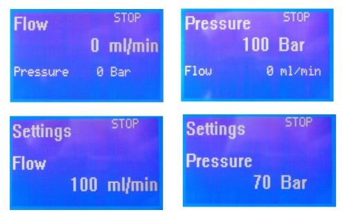
After switching on the pump is set to display the first item. In the upper right corner shows the status of the pump (at this moment, STOP). The display shows the current flow and the current pressure. After pressing the F1 key to get to the second operating item display, where it is displayed as the current primary pressure and secondary current flow.
