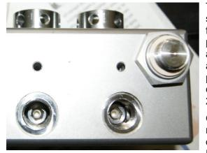
Fig. 7: Hexagonal caps and valves inside head, back side tighting screws
