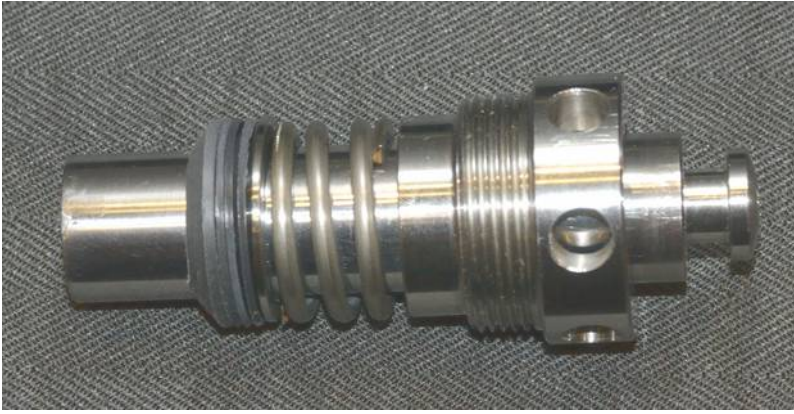
Fig. 3: Piston with sealings, spring and through bolt
