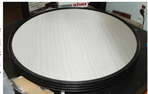
Fig. 7: Frit in the piston
