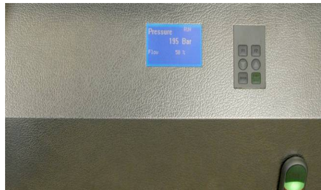
Fig. 14: Oil control display and keyboard
