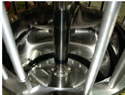
Fig. 9: Hydraulic piston with connecting flange and tube
