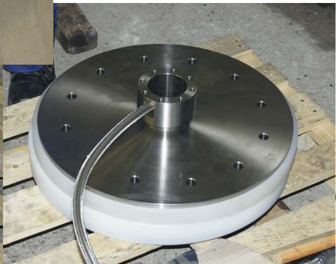
Fig. 10: Upper piston with flexible pipe, sealing ring, supporting ring, supporting plate and connecting tube
