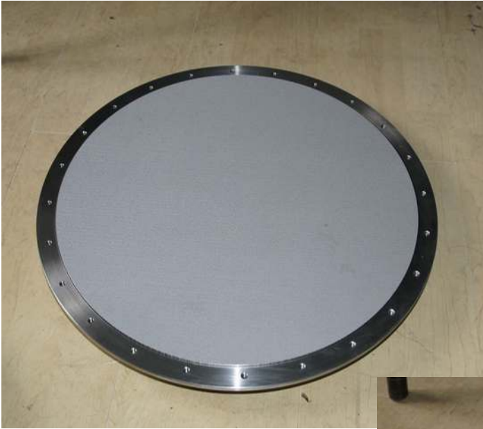
Fig. 8: Bottom piston with sealing ring
