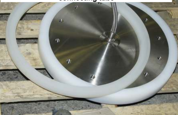
Fig. 10: Upper piston with flexible pipe, sealing ring, supporting ring, supporting plate and connecting tube
