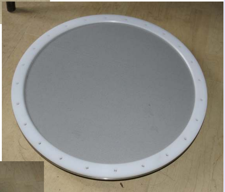
Fig. 8: Bottom piston with sealing ring
