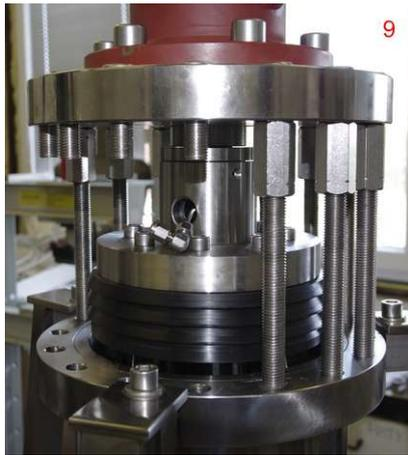
Support rods are completed by leg support plate made of 5 mm thick steel connected to rods by 6 sleeves On one leg are connected panel for flow reversion and UV detector remote cell (Fig 12, 13). Both panels are connected to the leg by bolts M6.
