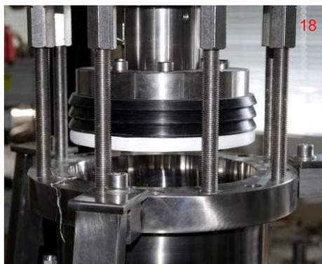
Hydraulic piston is moved down carefully to reach the smallest gap between CP 11 and CP 2. Three bolts on CP 2 have to be released during this procedure and they are slightly tightened when CP 1 is inside the groove on upper part of CP 2. The whole is moved a bit up and metal sheet is removed.
