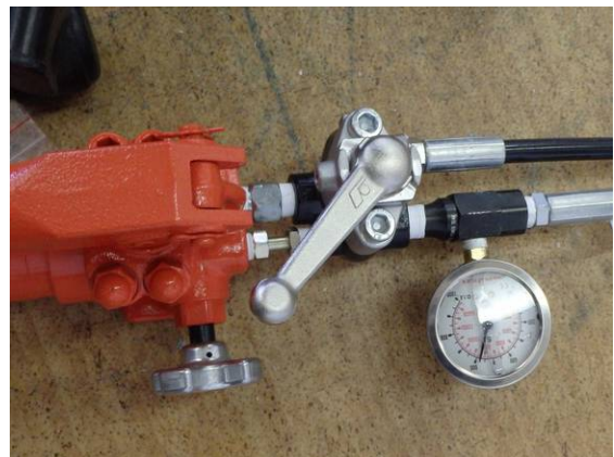
Fig. 9 Oil pump head with switching valve
