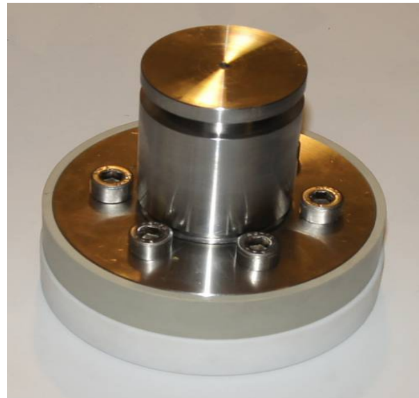
Fig. 6 Upper piston with support plate and connecting piece 1
