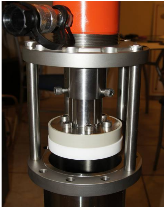
Fig. 8 Upper piston inserted on its position, connecting pieces fixed
