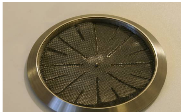
Fig. 4 Frit ring with distributor nets
